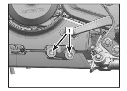
Remove the oil filter cover 2 and replace the old oil filter with a new oil filter.
