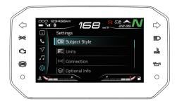
For Main interface: press it to switch Optional Info 1 and long press it to reset trips.
