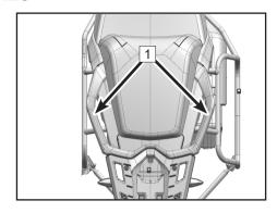
Footrests 2 are mounted on the motorcycle for the operator and passenger.
