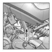
1 VIN NO. 2 Engine serial NO. 3 Name plate
