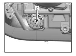
Remove oil filling plug and o-ring 3.
