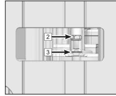
10. Remove the funnel assembly. Verify the oil level is between the upper and lower mark with the dipstick, and adjust the oil level accordingly.
