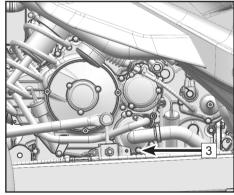
9. During filling coolant, unscrew the coolant drain bolt to release residual air inside the coolant hose until only fluid flows out, then screw back in and tighten the drain bolt.
