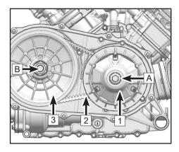
The secondary clutch (3) is mounted to the input shaft of the transmission (B) and serves two functions. As a "slave" pulley to the primary clutch, and to provide a torque sensing element that shifts drive ratios. The drive belt (2) is a heavy duty V-belt that connects the engine and transmission clutch pulleys.
