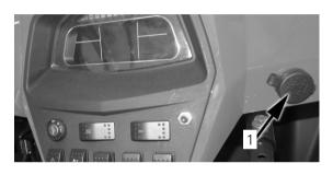
1. 12V DC outletThis vehicle has 1 DC outlet.Output voltage:12 VMaximum output current: 10 A
