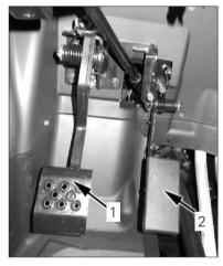
1. Brake pedal 2. Throttle pedal
