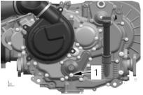
1. Coolant drain bolt
