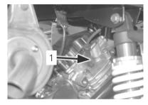
1. Spark plug cap, front cylinder
