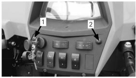
1. SET button 2. Clock button To reset the clock:
