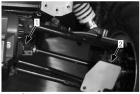
1. Inner CV joint 2. Outer CV joint
