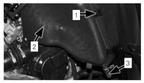
1. Clamp 2. Air filter cover 3. Moisture catch tube
